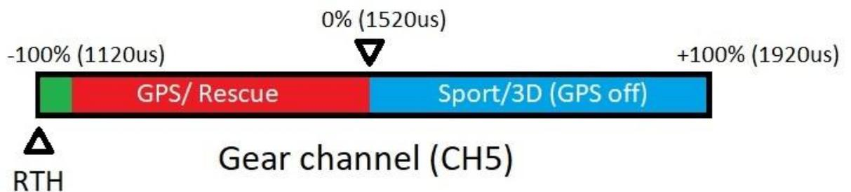
**Transmitter setting for GPS flight mode:** Set channel 5 of transmitter to negative value (less than center 1520us) for GPS flight mod. Value range from -90% to 0.
