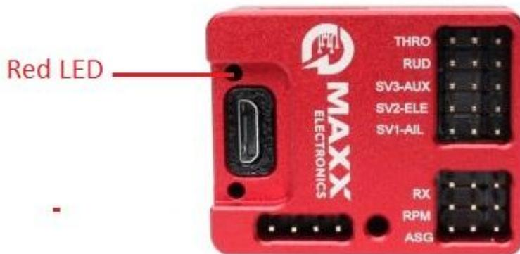
See the Red LED (on MAXX Flybarless unit, not the LED on GPS unit) status table:
